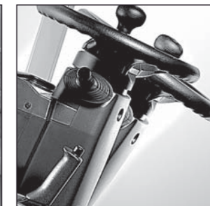
Adjustable steering column
