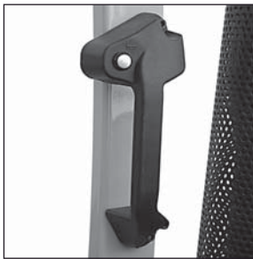
Grip/horn for reversing (optional)
