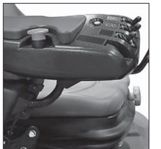
Fingertip hydraulic controls (optional)
